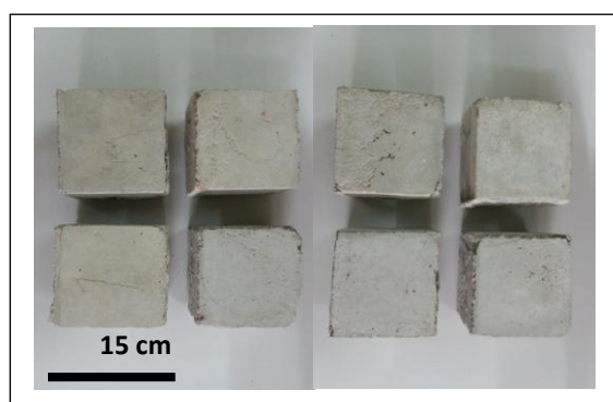
Figure-4: The concrete briquettes prepared from the studied limestones, in the different ratios of raw materials and water.
